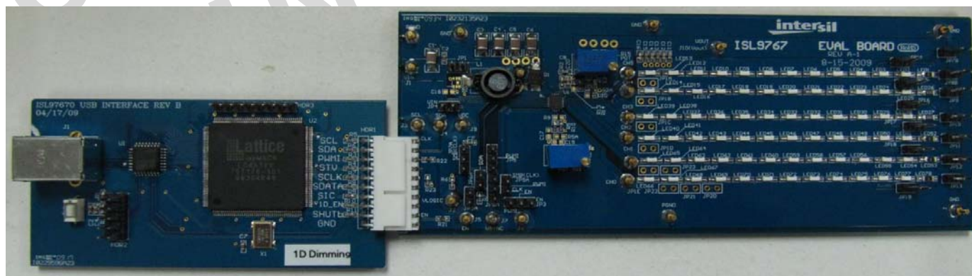
FIGURE 2. I 2 C INTERFACE BOARD CONNECTED TO ISL97671/2/3/4IRZ-EVAL EVALUATION BOARD
